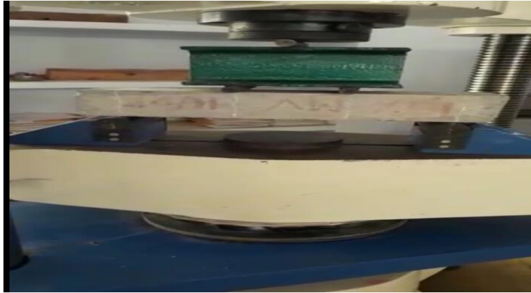
Fig. 4: Flexural strength testing set up
