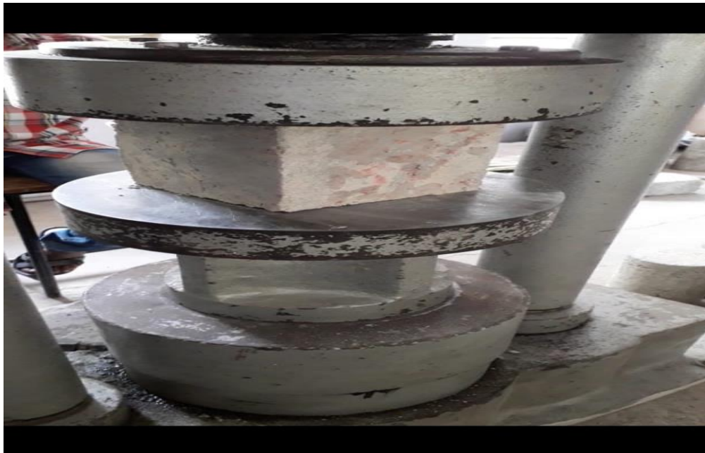
Fig. 2: Compressive strength testing set up
