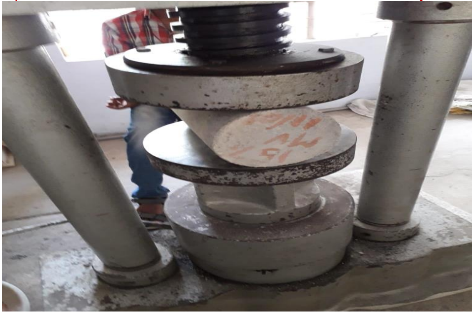
Fig 3: Tensile strength setting setup
